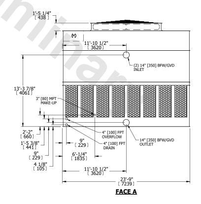
DRAWN BY: TAM NO. OF SHIPPING SECTIONS **SHIPPING** OPERATING HEAVIEST SECTION 20370 lbs+ [9240] kg+ 14100 lbs+ [6400] kg+ 36220 lbs+ [16430] kg+ WEIGHT WEIGHT WEIGHT
