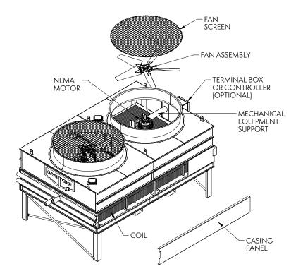
eco-Air Flat Coil Configuration with EC Fan Motors
