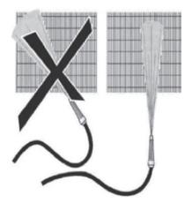
Figure 1 – Always Clean Fins in Vertical Direction
