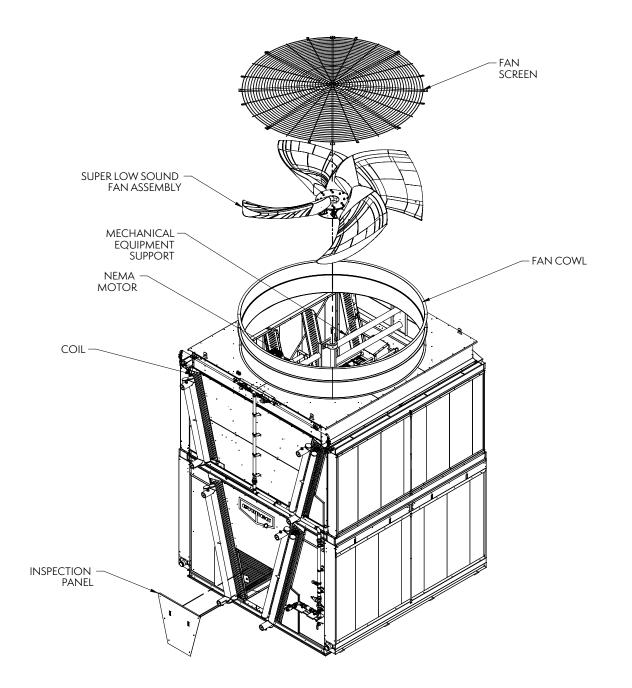
eco-Air Double Stack Adiabatic Cooler with NEMA Fan Motors and Optional Super Low Sound Fans
