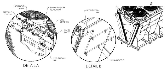
NOTE: If the adiabatic pad or spray pre-cooling system is provided with the "two-stage" accessory, quantity (2) solenoid valves will be provided.
