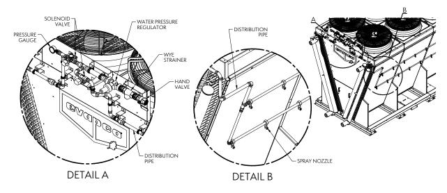
Figure 3 – Spray Pre-Cooling System Components
