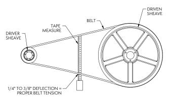
Figure 5 — Method 2, Measuring Fan Belt Deflection
