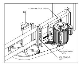
Figure 6 — Internally Mounted Motor, Double Stack
