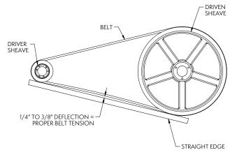
Figure 4 — Method 1, Measuring Fan Belt Deflection
