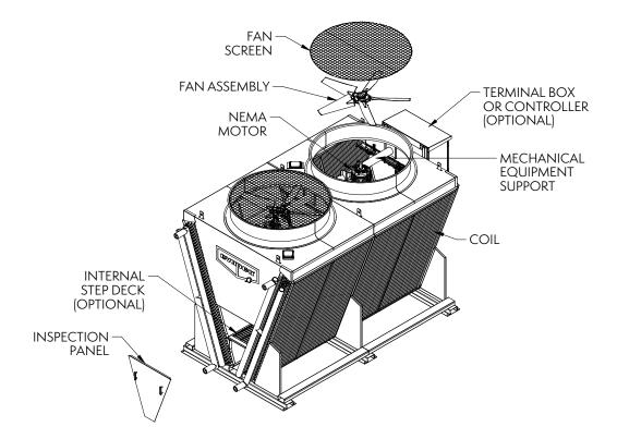
eco-Air V-Coil Configuration with EC Fan Motors
