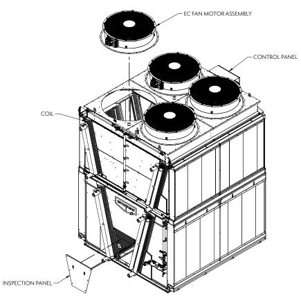
eco-Air Double Stack Adiabatic Cooler with EC Fan Motors
