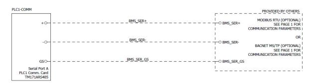
Figure 2 - Modbus RTU OR BACnet MS/TP Wiring Diagram
