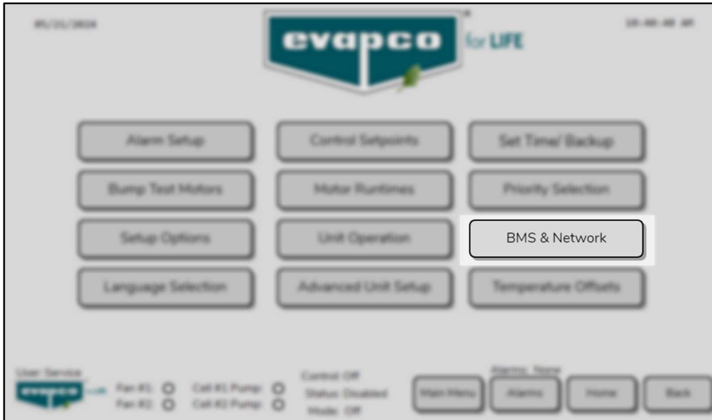
Figure 7 – Operator Menu, BMS & Network
