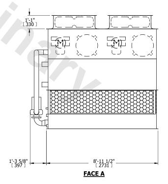
DRAWN BY: NO. OF SHIPPING SECTIONS **SHIPPING OPERATING** HEAVIEST SECTION 4110 lbs+ [1865] kg+ 3440 lbs+ [1565] kg+ 5820 lbs+ [2640] kg+ WEIGHT WEIGHT WEIGHT
