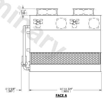
DRAWN BY: CAF NO. OF SHIPPING SECTIONS **SHIPPING** OPERATING HEAVIEST SECTION 6490 lbs+ [2945] kg+ 8860 lbs+ [4020] kg+ 5670 lbs+ [2575] kg+ WEIGHT WEIGHT WEIGHT
