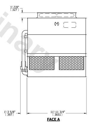
DRAWN BY: SLR NO. OF SHIPPING SECTIONS **SHIPPING** OPERATING HEAVIEST SECTION 13290 lbs+ [6030] kg+ 11490 lbs+ [5215] kg+ 17590 lbs+ [7980] kg+ WEIGHT WEIGHT WEIGHT
