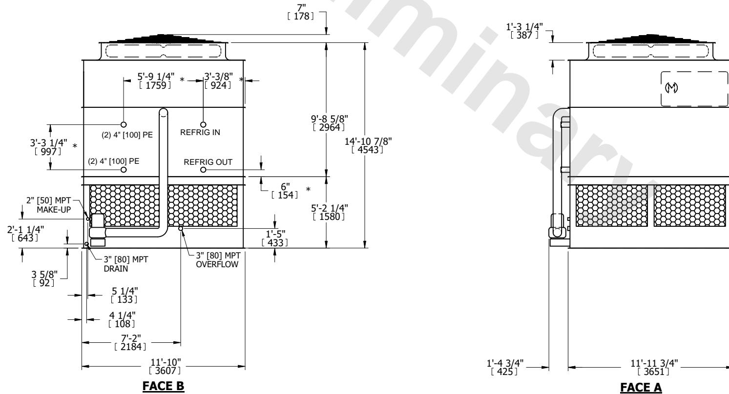
SHIPPING WEIGHT 18880 lbs+ [8565] kg+ OPERATING WEIGHT 25860 lbs+ [11730] kg+ HEAVIEST SECTION WEIGHT 16170 lbs+ [7335] kg+ NO. OF SHIPPING SECTIONS 2 DRAWN BY: SLR
