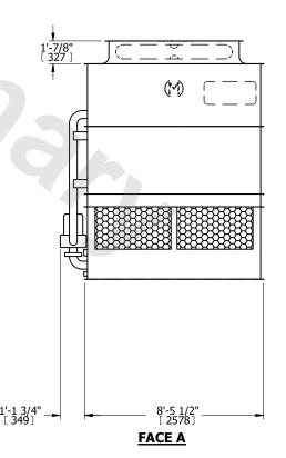
DRAWN BY: SLR NO. OF SHIPPING SECTIONS **SHIPPING OPERATING** HEAVIEST SECTION 6430 lbs+ [2920] kg+ 7730 lbs+ [3510] kg+ 10330 lbs+ [4690] kg+ WEIGHT WEIGHT WEIGHT
