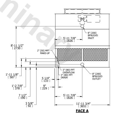
DRAWN BY: JLG SHIPPING NO. OF SHIPPING SECTIONS OPERATING HEAVIEST SECTION 5720 lbs+ [2595] kg+ 9580 lbs+ [4350] kg+ 3960 lbs+ [1800] kg+ WEIGHT WEIGHT WEIGHT
