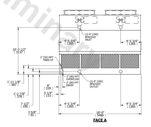
SHIPPING WEIGHT 9600 lbs+ [4355] kg+ OPERATING WEIGHT 15490 lbs+ [7030] kg+ HEAVIEST SECTION WEIGHT 6780 lbs+ [3080] kg+ NO. OF SHIPPING SECTIONS 2 DRAWN BY: JLG
