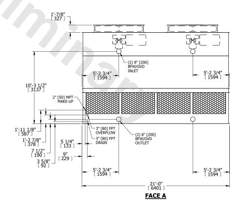
SHIPPING WEIGHT 11030 lbs+ [5005] kg+ OPERATING WEIGHT 17970 lbs+ [8155] kg+ HEAVIEST SECTION WEIGHT 7840 lbs+ [3560] kg+ NO. OF SHIPPING SECTIONS 2 DRAWN BY: JLG
