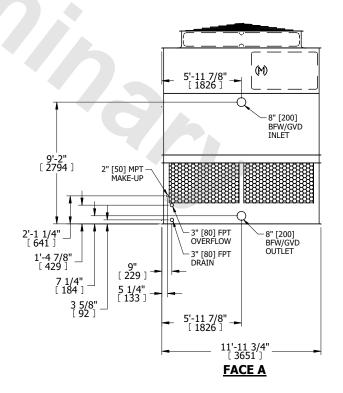
DRAWN BY: KDS NO. OF SHIPPING SECTIONS **SHIPPING** OPERATING HEAVIEST SECTION 7990 lbs+ [3625] kg+ 14200 lbs+ [6445] kg+ 5590 lbs+ [2540] kg+ WEIGHT WEIGHT WEIGHT
