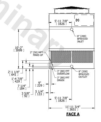
NO. OF SHIPPING SECTIONS **SHIPPING** OPERATING HEAVIEST SECTION 8880 lbs+ [4030] kg+ 6480 lbs+ [2940] kg+ 15090 lbs+ [6845] kg+ WEIGHT WEIGHT WEIGHT
