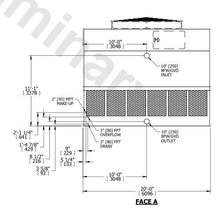
SHIPPING WEIGHT 13430 lbs+ [6095] kg+ OPERATING WEIGHT 23830 lbs+ [10810] kg+ HEAVIEST SECTION WEIGHT 9320 lbs+ [4230] kg+ NO. OF SHIPPING SECTIONS 2 DRAWN BY: KDS
