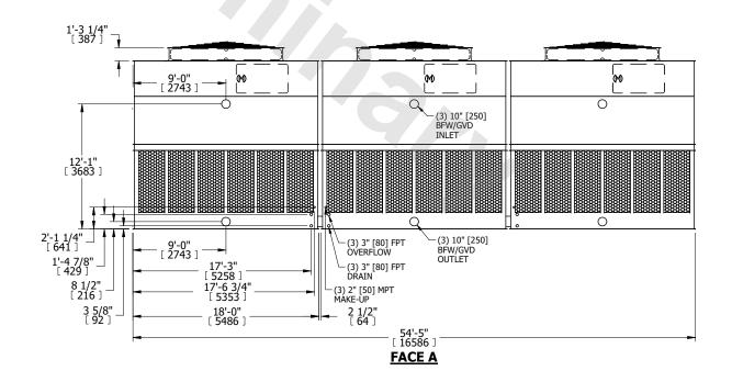
SHIPPING WEIGHT 35310 lbs+ [16020] kg+ OPERATING WEIGHT 63120 lbs+ [28635] kg+ HEAVIEST SECTION WEIGHT 7590 lbs+ [3445] kg+ NO. OF SHIPPING SECTIONS 6 DRAWN BY: KDS
