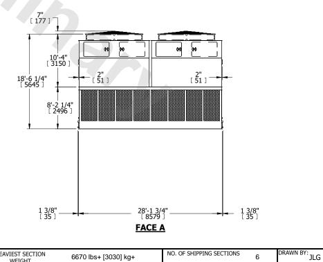
NO. OF SHIPPING SECTIONS **SHIPPING** OPERATING HEAVIEST SECTION 6670 lbs+ [3030] kg+ 39780 lbs+ [18045] kg+ 68680 lbs+ [31155] kg+ WEIGHT WEIGHT WEIGHT
