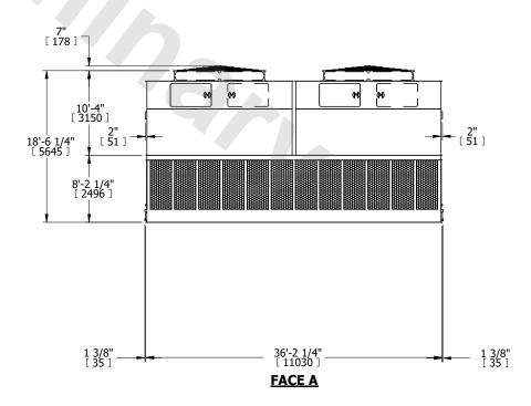
SHIPPING WEIGHT 52080 lbs+ [23625] kg+ OPERATING WEIGHT 88780 lbs+ [40270] kg+ HEAVIEST SECTION WEIGHT
