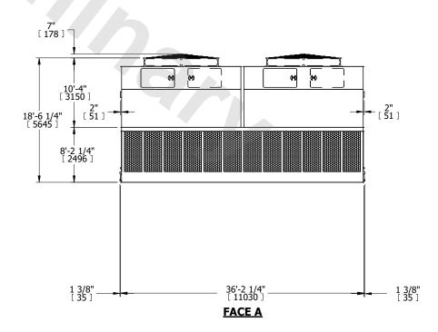
SHIPPING WEIGHT 52520 lbs+ [23825] kg+ OPERATING WEIGHT 89220 lbs+ [40470] kg+ HEAVIEST SECTION WEIGHT 8870 lbs+ [4025] kg+ NO. OF SHIPPING SECTIONS 6 DRAWN BY: KDS
