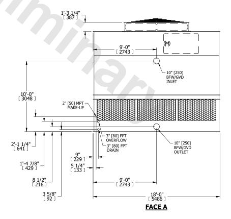
SHIPPING WEIGHT 10580 lbs+ [4800] kg+ OPERATING WEIGHT 18180 lbs+ [8250] kg+ HEAVIEST SECTION WEIGHT 7030 lbs+ [3190] kg+ NO. OF SHIPPING SECTIONS 2 DRAWN BY: KDS
