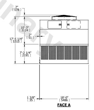
SHIPPING WEIGHT 22280 lbs+ [10110] kg+ OPERATING WEIGHT 37480 lbs+ [17005] kg+ HEAVIEST SECTION WEIGHT 7230 lbs+ [3280] kg+ NO. OF SHIPPING SECTIONS 4 DRAWN BY: KDS
