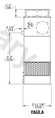
SHIPPING WEIGHT 1160 lbs+ [530] kg+ OPERATING WEIGHT 1790 lbs+ [815] kg+ HEAVIEST SECTION WEIGHT 810 lbs+ [370] kg+ NO. OF SHIPPING SECTIONS 2 DRAWN BY: KWC
