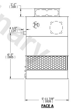
DRAWN BY: KWC NO. OF SHIPPING SECTIONS **SHIPPING** OPERATING HEAVIEST SECTION 1390 lbs+ [635] kg+ 2410 lbs+ [1095] kg+ 950 lbs+ [435] kg+ WEIGHT WEIGHT WEIGHT
