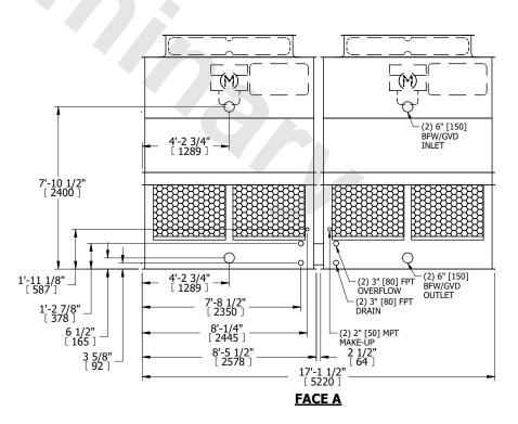
SHIPPING WEIGHT 7180 lbs+ [3260] kg+ OPERATING WEIGHT 12020 lbs+ [5455] kg+ HEAVIEST SECTION WEIGHT 2280 lbs+ [1035] kg+ NO. OF SHIPPING SECTIONS 4 DRAWN BY:
