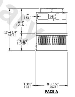
SHIPPING WEIGHT 7320 lbs+ [3325] kg+ OPERATING WEIGHT 12160 lbs+ [5520] kg+ HEAVIEST SECTION WEIGHT 2320 lbs+ [1055] kg+ NO. OF SHIPPING SECTIONS 4 DRAWN BY: JLG
