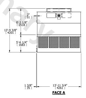
SHIPPING WEIGHT 12760 lbs+ [5790] kg+ OPERATING WEIGHT 21780 lbs+ [9880] kg+ HEAVIEST SECTION WEIGHT 4240 lbs+ [1925] kg+ NO. OF SHIPPING SECTIONS 4 DRAWN BY: KDS
