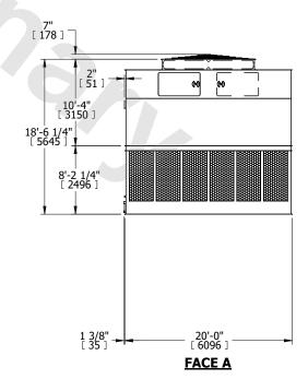
DRAWN BY: KDS NO. OF SHIPPING SECTIONS **SHIPPING** OPERATING HEAVIEST SECTION 27760 lbs+ [12595] kg+ 9260 lbs+ [4205] kg+ 48560 lbs+ [22030] kg+ WEIGHT WEIGHT WEIGHT
