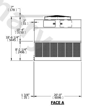
DRAWN BY: KDS NO. OF SHIPPING SECTIONS **SHIPPING** OPERATING HEAVIEST SECTION 27880 lbs+ [12650] kg+ 9320 lbs+ [4230] kg+ 48680 lbs+ [22085] kg+ WEIGHT WEIGHT WEIGHT
