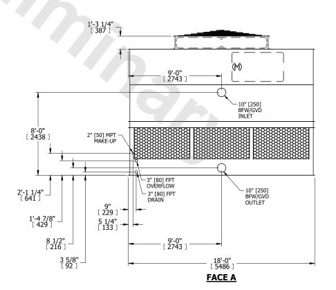
DRAWN BY: KDS NO. OF SHIPPING SECTIONS **SHIPPING** OPERATING HEAVIEST SECTION 9260 lbs+ [4205] kg+ 16860 lbs+ [7650] kg+ 5710 lbs+ [2595] kg+ WEIGHT WEIGHT WEIGHT
