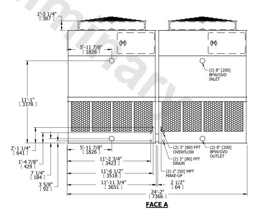
SHIPPING WEIGHT 15320 lbs+ [6950] kg+ OPERATING WEIGHT 25240 lbs+ [11450] kg+ HEAVIEST SECTION WEIGHT 5220 lbs+ [2370] kg+ NO. OF SHIPPING SECTIONS 4 DRAWN BY: JLG
