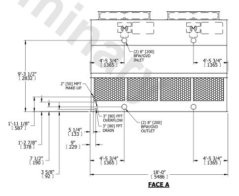
SHIPPING WEIGHT 8720 lbs+ [3960] kg+ OPERATING WEIGHT 14610 lbs+ [6630] kg+ HEAVIEST SECTION WEIGHT 5900 lbs+ [2680] kg+ NO. OF SHIPPING SECTIONS 2 DRAWN BY: JLG
