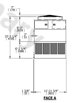
SHIPPING WEIGHT 14260 lbs+ [6470] kg+ OPERATING WEIGHT 24180 lbs+ [10970] kg+ HEAVIEST SECTION WEIGHT 4680 lbs+ [2125] kg+ NO. OF SHIPPING SECTIONS 4 DRAWN BY: KDS
