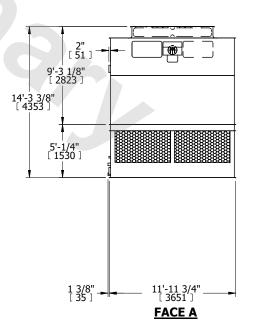
SHIPPING WEIGHT 12400 lbs+ [5625] kg+ OPERATING WEIGHT 20120 lbs+ [9130] kg+ HEAVIEST SECTION WEIGHT 4350 lbs+ [1975] kg+ NO. OF SHIPPING SECTIONS 4 DRAWN BY: KDS
