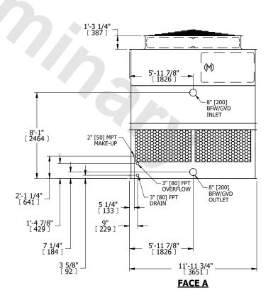
SHIPPING WEIGHT 6620 lbs+ [3005] kg+ OPERATING WEIGHT 11580 lbs+ [5255] kg+ HEAVIEST SECTION WEIGHT 4200 lbs+ [1910] kg+ NO. OF SHIPPING SECTIONS 2 DRAWN BY: JLG
