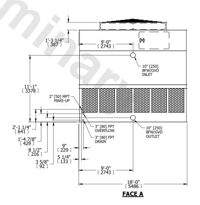
SHIPPING NO. OF SHIPPING SECTIONS OPERATING HEAVIEST SECTION 12120 lbs+ [5500] kg+ 21390 lbs+ [9705] kg+ 8220 lbs+ [3730] kg+ WEIGHT WEIGHT WEIGHT
