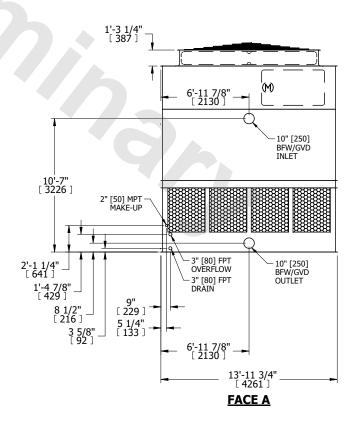
SHIPPING WEIGHT 9410 lbs+ [4270] kg+ OPERATING WEIGHT 16740 lbs+ [7595] kg+ HEAVIEST SECTION WEIGHT 6540 lbs+ [2970] kg+ NO. OF SHIPPING SECTIONS 2 DRAWN BY: KDS
