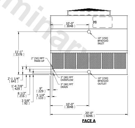
SHIPPING WEIGHT 13000 lbs+ [5900] kg+ OPERATING WEIGHT 23400 lbs+ [10615] kg+ HEAVIEST SECTION WEIGHT 8890 lbs+ [4035] kg+ NO. OF SHIPPING SECTIONS 2 DRAWN BY: KDS
