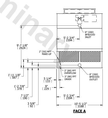
SHIPPING WEIGHT 5330 lbs+ [2420] kg+ OPERATING WEIGHT 8630 lbs+ [3915] kg+ HEAVIEST SECTION WEIGHT 3730 lbs+ [1695] kg+ NO. OF SHIPPING SECTIONS 2 DRAWN BY:
