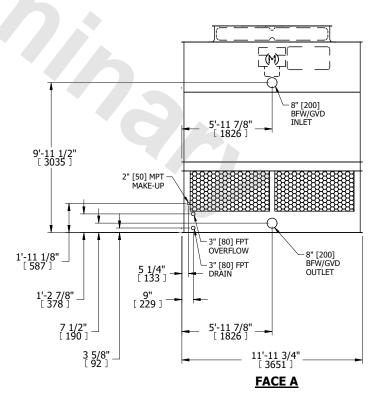
SHIPPING WEIGHT 5940 lbs+ [2695] kg+ OPERATING WEIGHT 9800 lbs+ [4450] kg+ HEAVIEST SECTION WEIGHT 4180 lbs+ [1900] kg+ NO. OF SHIPPING SECTIONS 2 DRAWN BY: JLG
