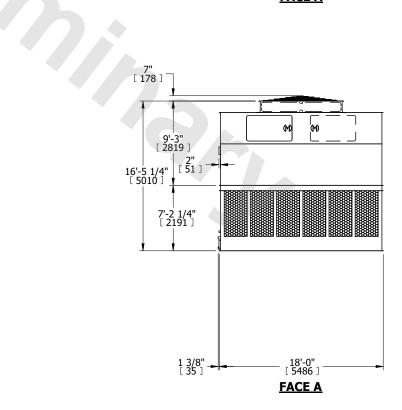
SHIPPING WEIGHT 20480 lbs+ [9290] kg+ OPERATING WEIGHT 35680 lbs+ [16185] kg+ HEAVIEST SECTION WEIGHT 6330 lbs+ [2875] kg+ NO. OF SHIPPING SECTIONS 4 DRAWN BY: JLG
