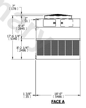
SHIPPING WEIGHT 23720 lbs+ [10760] kg+ OPERATING WEIGHT 42260 lbs+ [19170] kg+ HEAVIEST SECTION WEIGHT 7480 lbs+ [3395] kg+ NO. OF SHIPPING SECTIONS 4 DRAWN BY: KDS
