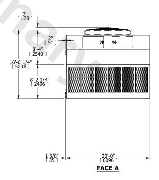
SHIPPING WEIGHT 23980 lbs+ [10880] kg+ OPERATING WEIGHT 44780 lbs+ [20315] kg+ HEAVIEST SECTION WEIGHT 7370 lbs+ [3345] kg+ NO. OF SHIPPING SECTIONS 4 DRAWN BY: BLL
