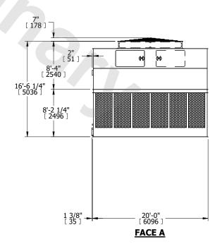
DRAWN BY: BLL NO. OF SHIPPING SECTIONS **SHIPPING** OPERATING HEAVIEST SECTION 24620 lbs+ [11170] kg+ 45420 lbs+ [20605] kg+ 7690 lbs+ [3490] kg+ WEIGHT WEIGHT WEIGHT
