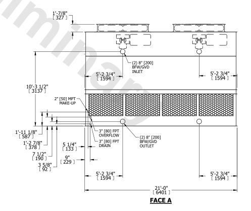
SHIPPING WEIGHT 10590 lbs+ [4805] kg+ OPERATING WEIGHT 17530 lbs+ [7955] kg+ HEAVIEST SECTION WEIGHT 7400 lbs+ [3360] kg+ NO. OF SHIPPING SECTIONS 2 DRAWN BY: JLG
