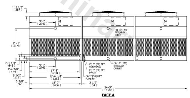
SHIPPING WEIGHT 32640 lbs+ [14810] kg+ OPERATING WEIGHT 60450 lbs+ [27420] kg+ HEAVIEST SECTION WEIGHT 6700 lbs+ [3040] kg+ NO. OF SHIPPING SECTIONS 6 DRAWN BY: KDS
