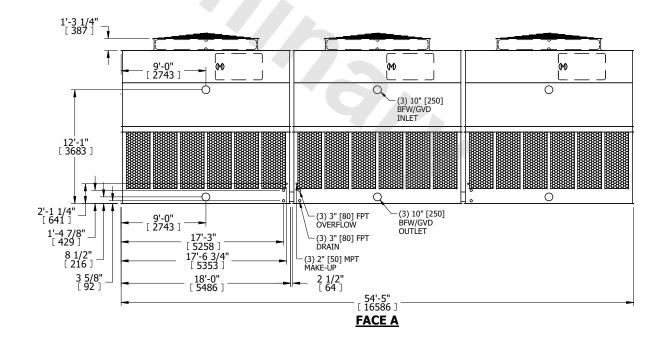
SHIPPING WEIGHT 34980 lbs+ [15870] kg+ OPERATING WEIGHT 62790 lbs+ [28485] kg+ HEAVIEST SECTION WEIGHT 7480 lbs+ [3395] kg+ NO. OF SHIPPING SECTIONS 6 DRAWN BY: KDS
