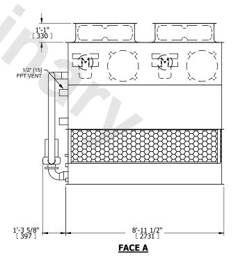
DRAWN BY: NO. OF SHIPPING SECTIONS **SHIPPING** OPERATING HEAVIEST SECTION 3440 lbs+ [1565] kg+ 4110 lbs+ [1865] kg+ 6310 lbs+ [2865] kg+ WEIGHT WEIGHT WEIGHT
