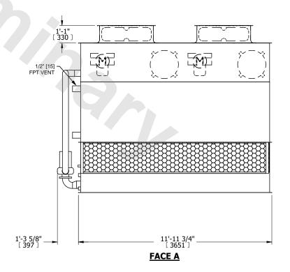
NO. OF SHIPPING SECTIONS **SHIPPING** OPERATING HEAVIEST SECTION 6430 lbs+ [2920] kg+ 9850 lbs+ [4470] kg+ 5610 lbs+ [2545] kg+ WEIGHT WEIGHT WEIGHT
