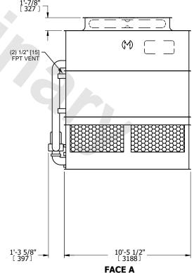
NO. OF SHIPPING SECTIONS **SHIPPING** OPERATING HEAVIEST SECTION 12210 lbs+ [5540] kg+ 17870 lbs+ [8110] kg+ 10570 lbs+ [4795] kg+ WEIGHT WEIGHT WEIGHT
