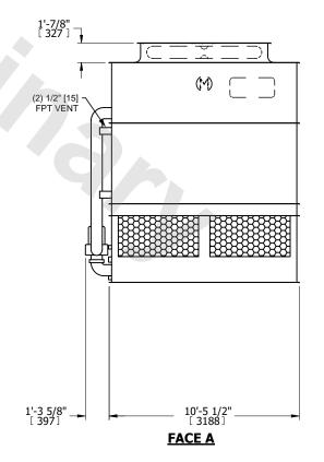
DRAWN BY: SLR NO. OF SHIPPING SECTIONS **SHIPPING OPERATING** HEAVIEST SECTION 12000 lbs+ [5445] kg+ 13640 lbs+ [6190] kg+ 19790 lbs+ [8980] kg+ WEIGHT WEIGHT WEIGHT
